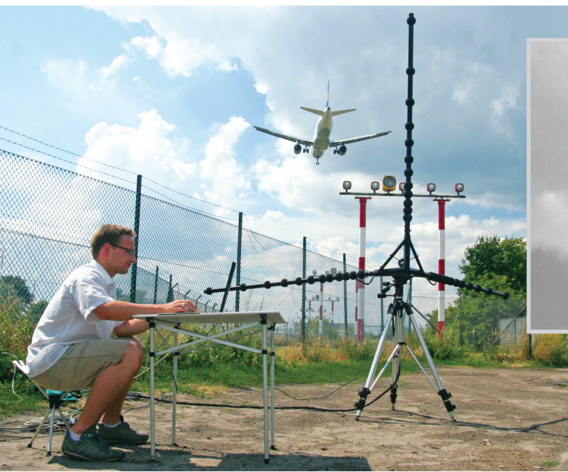
• • • Noise radiation from aircraft engines, gear and flaps and Acoustic Photo 2D.
